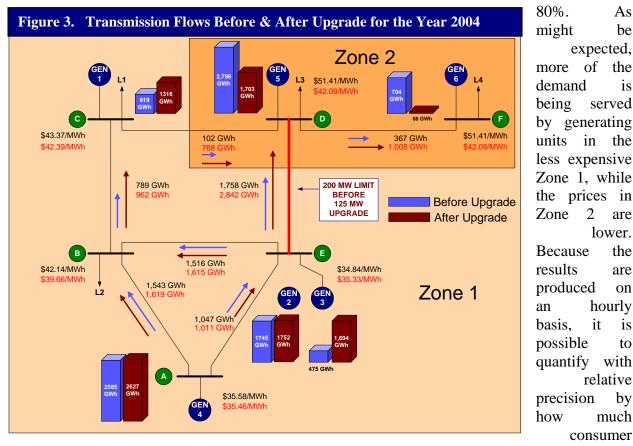
The changes in the generator performance for 2004 between the base case and the upgrade case are shown in Table 4. The annual load flows on each line before and after the
